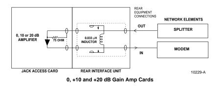
Figure 5. Access Jack, Amp Cards and RIU Schematic
